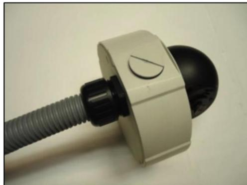
Adjust the viewing angle and focus of the camera and put the dome cover back on, and tighten it by using the screws.
