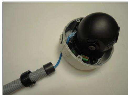
Push the head of the flex conduit, wrapped with sealing insert, into the body of the conduit gland.
