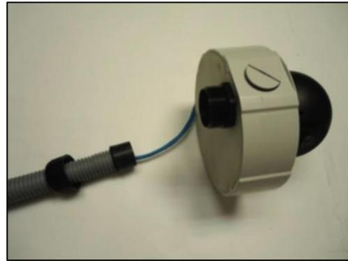
Connect the Ethernet cable to the camera's network port. If you are not using PoE, then please remember to pull the DC power cable through the flex conduit as well, and connect to the camera at this point.
